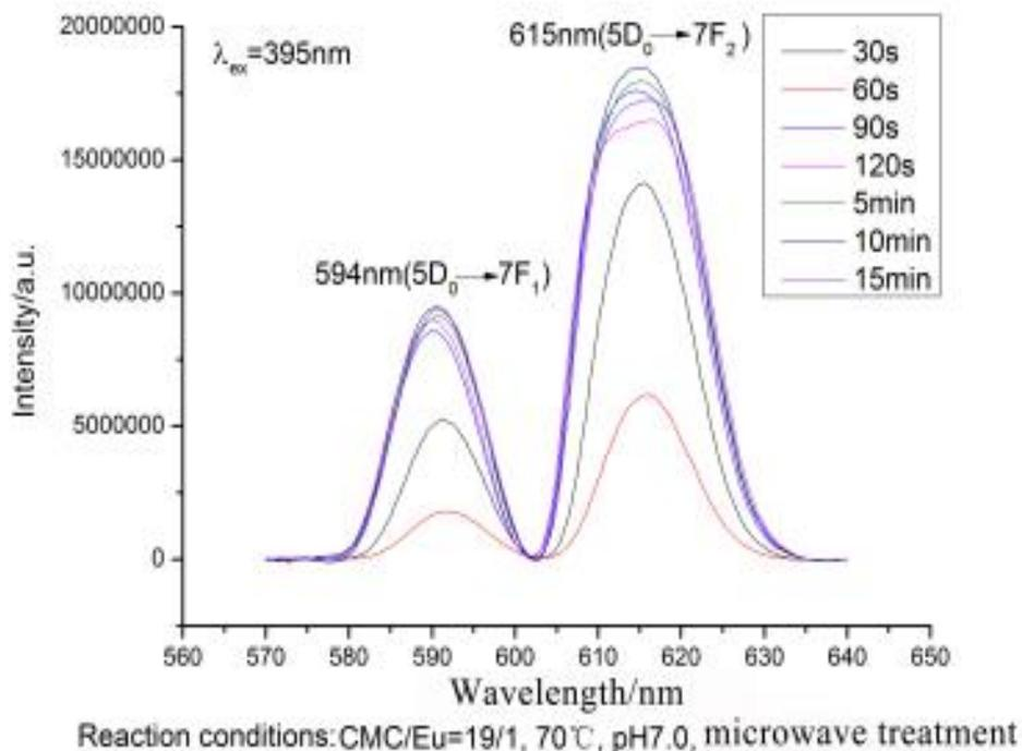
Figure the fluorescence spectra of CMC/Eu nanocomposites synthesized in different time
